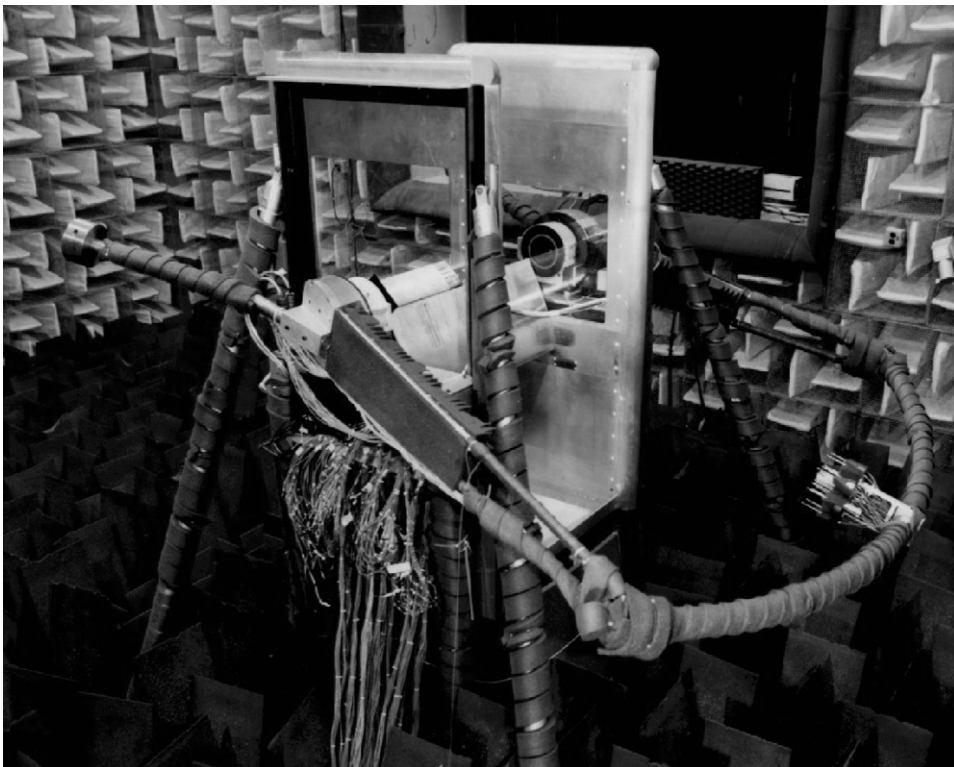
Fig. 1. Test apparatus with SADA mounted on pivotal boom in QFF.
